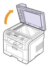
Place the original face down on the scanner glass and align it with the registration guide at the top left corner of the glass.
